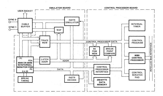
Figure 1. ICE-49 Module Block Diagram
